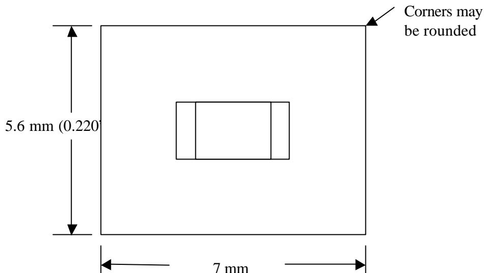
Circular holes can be used, but they would require a larger total cutout area, a diameter of 7 mm (0.275") to be certain. However, a 6.35 mm (0.250") diameter cutout is common for this size of LED, if your die-cutting and laminating processes are well registered. However, if your processes are not under control this may result in additional problems.
