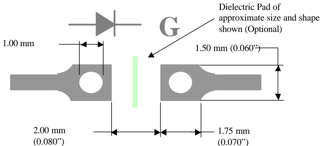
**LED Size and Style** – Nicomatic recommends that the largest possible LED be used to reduce the assembly cost of the LED. For most designs, the length and width of the part is not critical, only the height of the LED needs to be minimized. Utilizing LEDs with smaller length and width dimensions will increase the assembly cost. The standard LED used in the industry is the 1206 LED.
