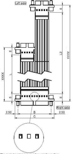
The main housing requires two empty cavities. Example: For a main housing of 22 pins, the two branches' housings will be 10pins and 10pins
