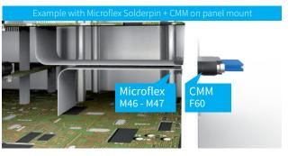
Reverse construction w/CMM on PCB + Microflex on panel mount possible. Please contact us.
