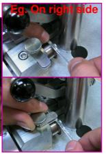
4. Place the 2 parallel strips onto the pins and stop the reel of contacts with the 1st bolt action on the right side. Then crimp as indicated on 5<sup>th</sup> step until the stop
