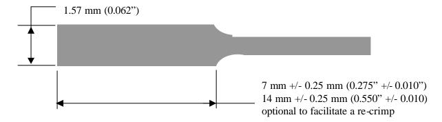
Note: When possible, the traces (circuit and dummy), should be designed 14 mm (0.550") long. This may allow the connector to be cut off and re-attached if it is mis-crimped, if this would be an acceptable repair for the end customer.
