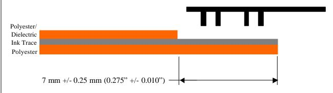
**B. Double Sided Circuit** – A dummy trace should be provided opposite the actual circuit. Ie. Opposite a trace on the top circuit there should be a dummy trace printed on the bottom circuit. The dummy trace should have a width of 1.57 mm (0.062") nominal and a length of 7 mm (0.275 "). This provides a thicker layer of ink to insure a reliable electrical connection. Note: There should be no adhesive or dielectric between the dummy trace and the active trace.
